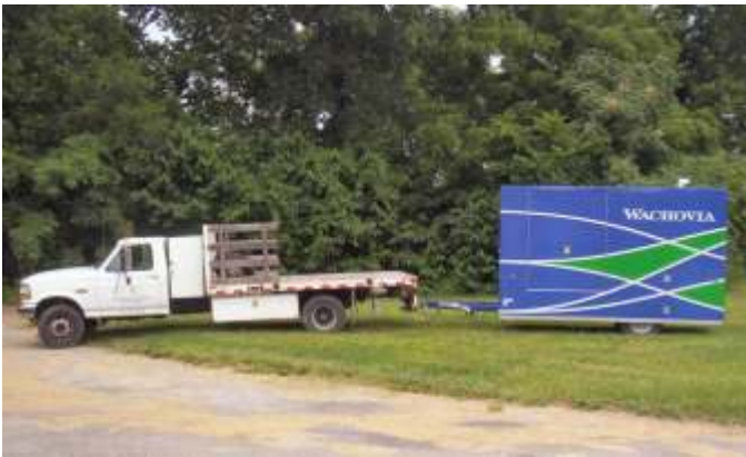
The Mobile ATM Kiosk may be towed using any truck with a 7,000 lb. towing capacity and a standard towing hitch.
