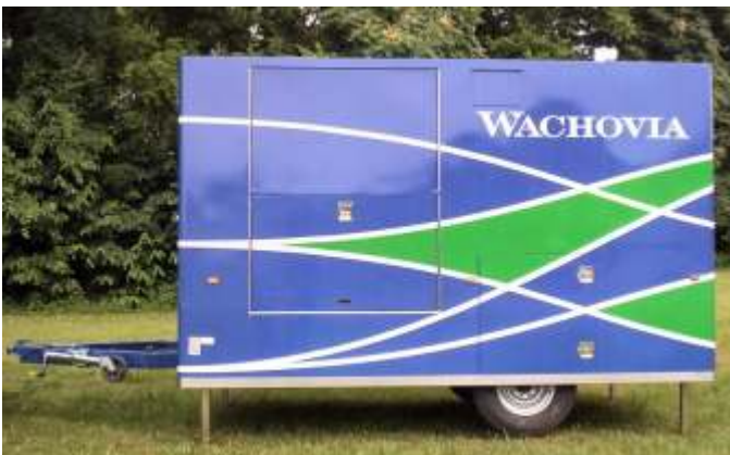
The Mobile Kiosk jacks are in place and the towing vehicle is unhooked. Now the towing tongue is ready to be stowed in its locking compartment.
