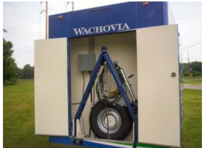
The towing tongue folds up into its locking cabinet.
