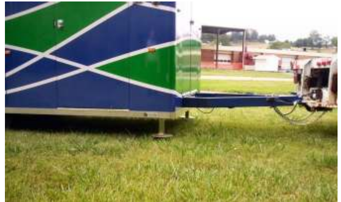
The Jack Stands are lowered using the remote control until all four jacks are touching the ground.
